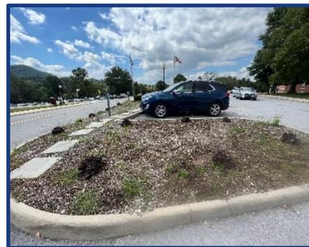
Figure 2.2: Facility lacks accessible route from parking area
