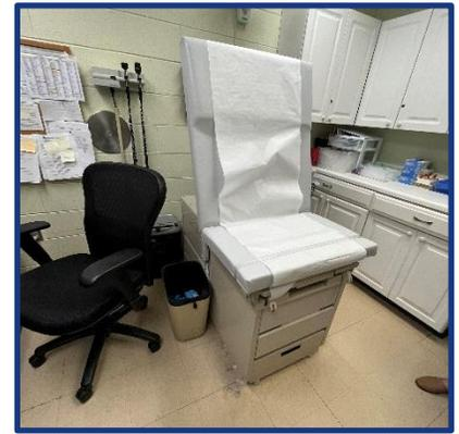
Figure 10: Lack of clear floor space and nonadjustable height exam chair
