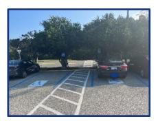
Figure 3.1: Low parking signs and inadequate access aisle width and location
